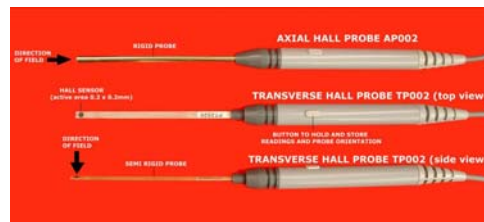
Figure 7. Axial and transverse Hall probes (Photo courtesy of Hirst Magnetic Instruments, Ltd.)
