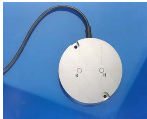
Figure 3. A pole cap, showing embedded pole coils (Photo courtesy of Magnet Physik Dr. Steingroever GmbH)
