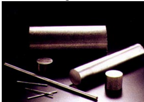
TERFENOL-D can be produced in specific shapes for a variety of applications.
